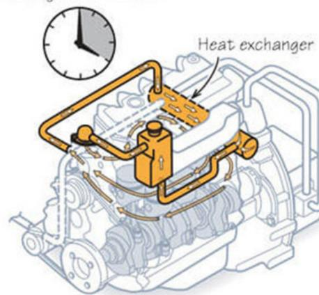
Start engine to circulate solution through internal cooling channels. Run engine intermittently on and off every 30 minutes for four hours.
