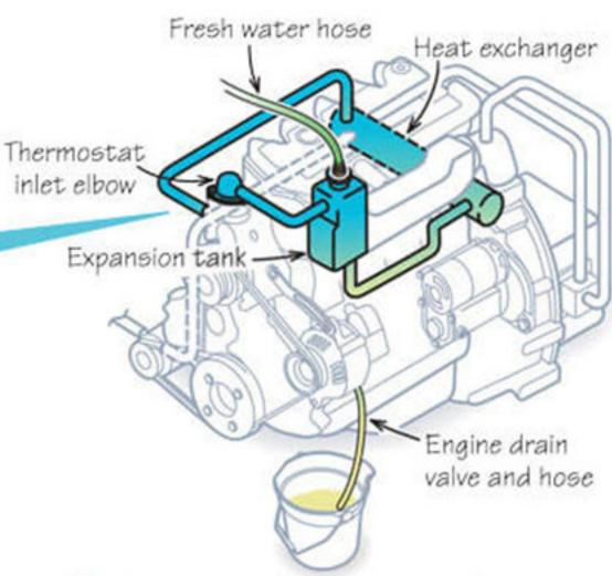
Drain coolant from engine and flush with fresh water to ensure all the coolant has been completely removed.
