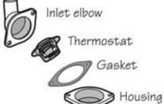
To ensure proper flow, remove the thermostat during the flushing procedure.
